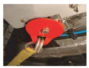
To install, unscrew bolt and slide the tab into the jacking block underneath the car. Make sure the tie downs are pointed towards the opposite side front wheel. Reinstall bolt
